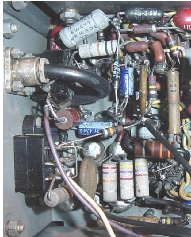
Replacement cathode by-pass caps and a few replacement resistors in the audio and IF cathode-follower stages
